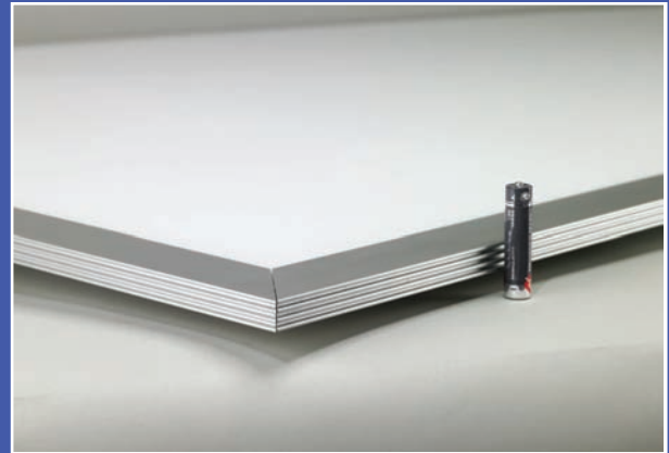
This 23.5" x 23.5" troffer downlight features a slim, lightweight backlight assembly that is edge lit with high efficiency LEDs that focus the light into a high-performance light guide.
